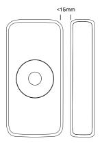
Remove the protective layer on the doublesided tape on the device (A). Place the device on the wall or door/window frame.
